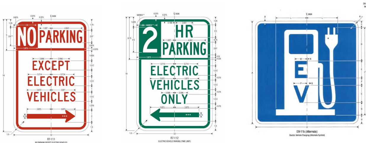
Figure 10. Examples of EV signage.
